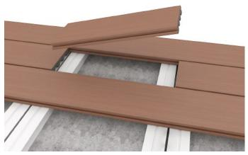
Place a new decking board of the same size into the groove, then secure it with screws as shown in the figure.
