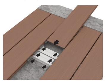
Replacement of the decking (installed with plastic clips) Case 2: I-shaped installation
