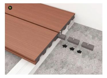
The plastic clips must be screwed vertically onto the joist, as shown in the figure.
